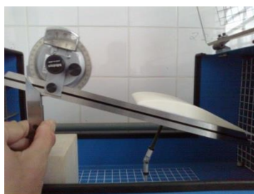
Figure 6. Method used to measure airfoil angles of attack (clockwise direction).
