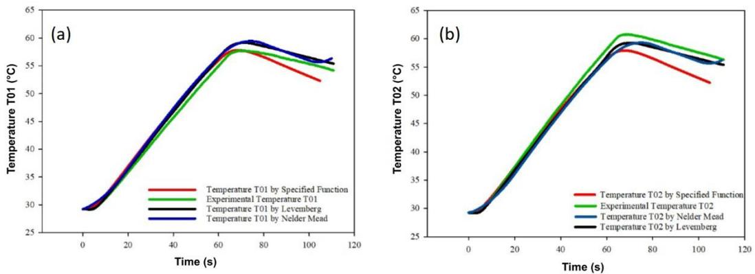
To emphasize the temperature comparison, the disparity between numerical and experimental data is depicted through Fig. 4(a) and Fig. 4(b). The deviations related to the
